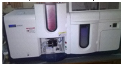
Atomic Absorption Spectrometer with flame and Graphite furnace (Hitachi ZA 3000)
