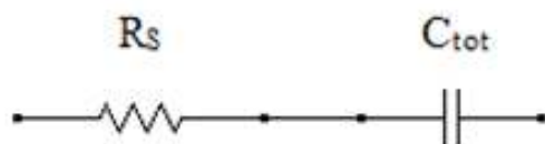
Figure 1: Randles equivalent circuit for a modified electrode without a redox mediator.
