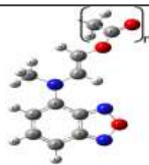
Fig. 9: Fluorescent temperature sensor With increasing temperature, about 40° C this compound gets fluorescent as green colour.
