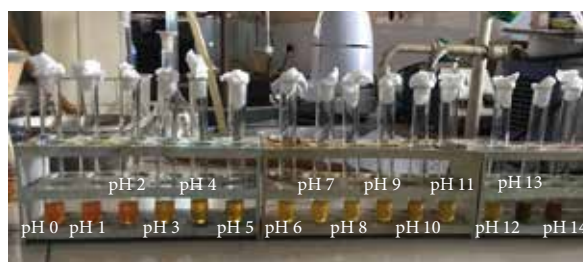
Figure 1: Change in colour of the methanolic extract of red catappa leaves with pH
